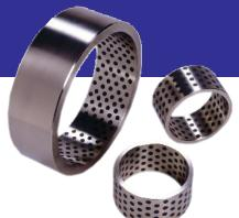
LUBRON® SL self-lubricating bearings are specifically designed to satisfy the demanding requirements of heavy duty industrial and structural applications. LUBRON SL bearings are available in a wide variety of bearing alloys, and employ solid lubricants compressed into trepanned or circular recesses for long-term lubrication.
